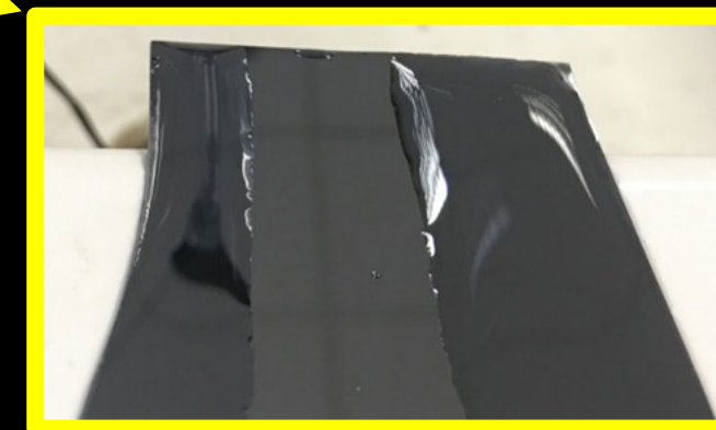
Hydrophobic surface due to ligand adsorption : NO SnO 2 deposition
